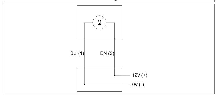
The assignment of the wires BU (1) and BN (2) according to the direction of travel is dependent on how the drive is installed (mounted to the right or to the left).
